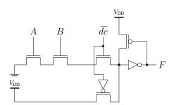
Figure 3: Transitions of SRDL mapped to LUT3
