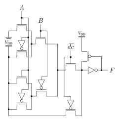
Figure 2: Single-Rail Domino Logic mapped to LUT3
